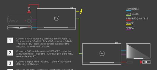
To control your HDMI source from your display location connect the IR TX to the 'IR (OUT)' port on the XTND transmitter (TX). Ensure that the IR TX is positioned over the IR window on your source device.
